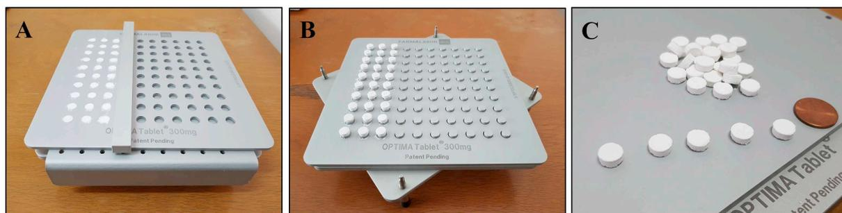
Fig. 2. Molding technique: (A) filled molds with wet powder blend; (B) ejection of the tablets from the molds; (C) sodium DCA tablets.
